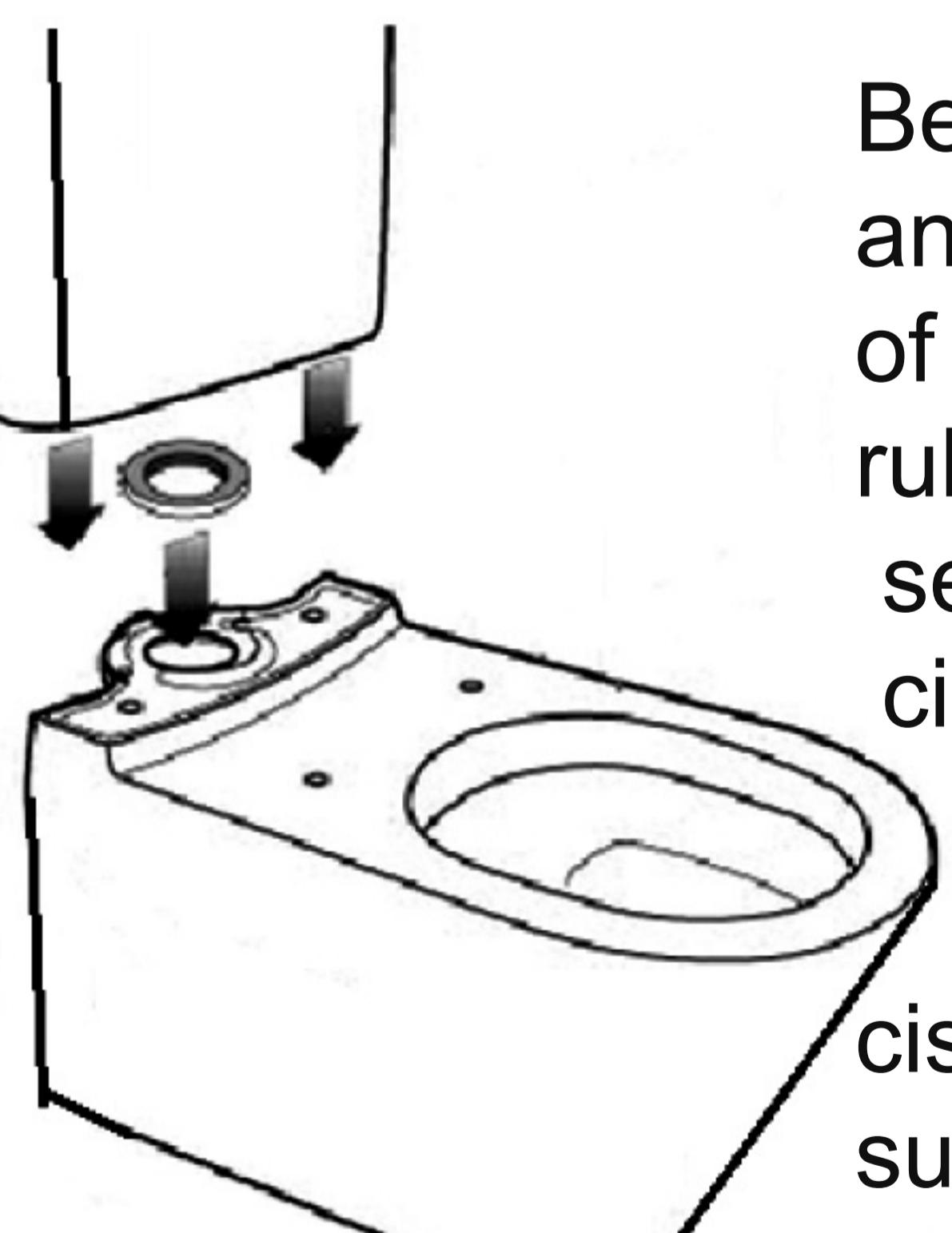
Before installing cistern, please check bungs and valves are tightened correctly. Put a bead of silicon to both upper and lower surfaces of foam rubber seal between cistern and pan. Place rubber seal at the bottom of the cistern, then gently lower cistern onto pan. Make sure the screws holes are matching between cistern and pan. Apply a beat of silicon around the bolts, then secure cistern to the pan. Before tightened fully make sure cistern sites square and straight to pan.
