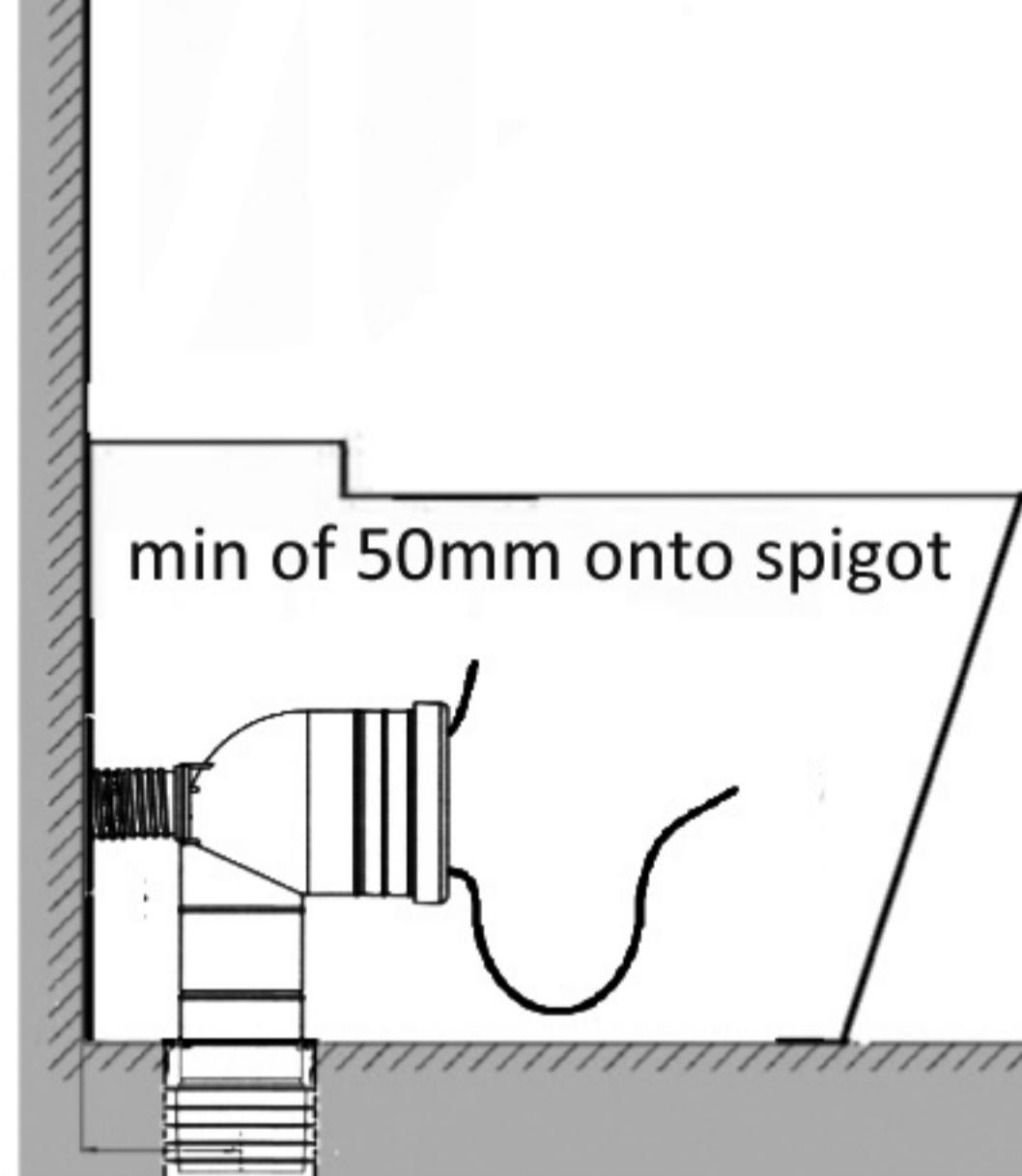
4. Align and push fully assembled toilet back to the wall
