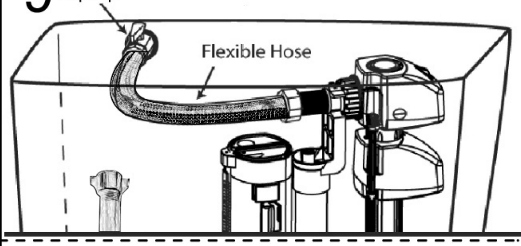
9. IF STEP 8 IS COMPLETED, SKIP THIS STEP. Fit off stop tap then connect rear water inlet valve to stop tap. Fill cistern and ensure correct water level.
