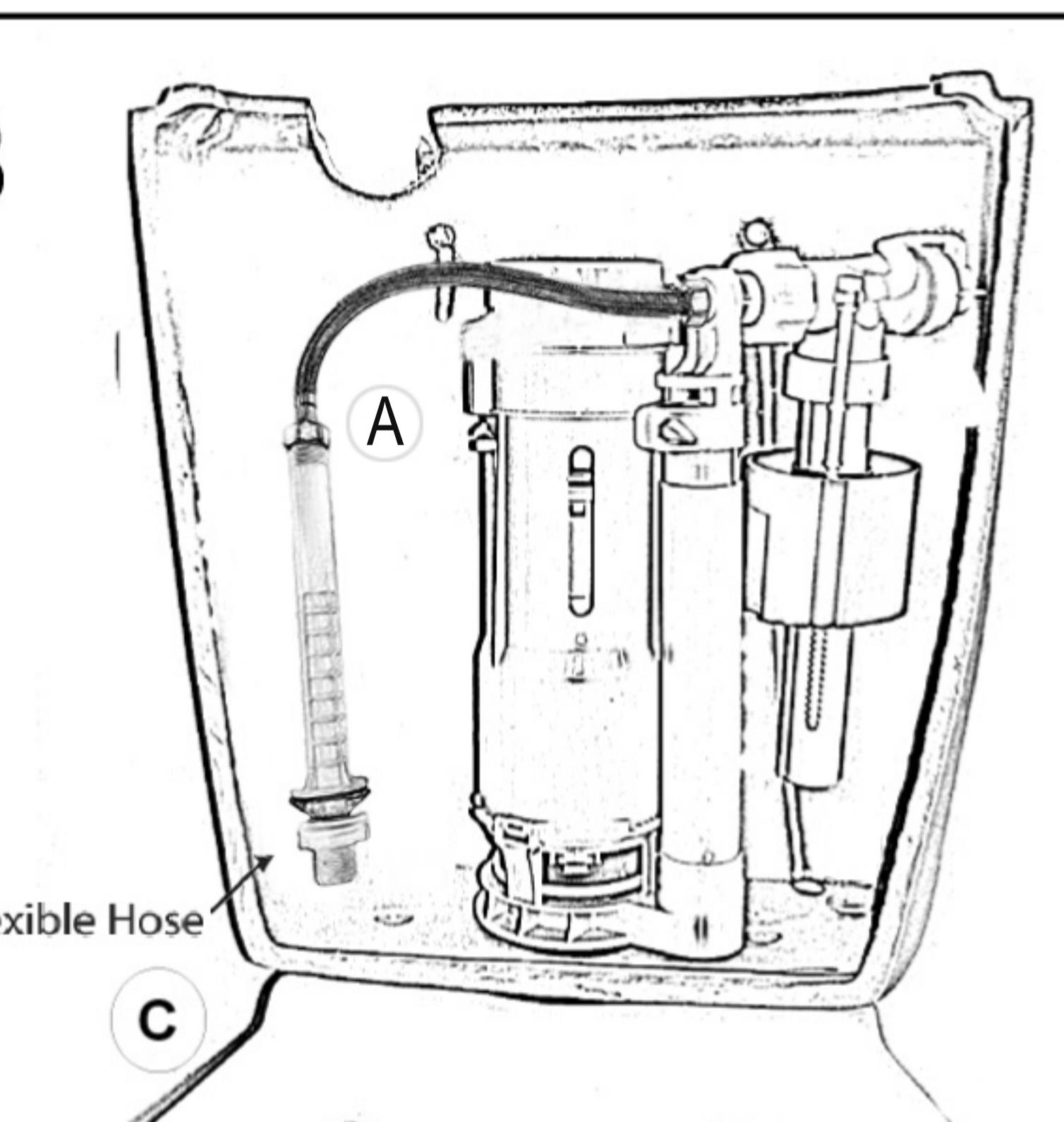
8. IF BACK INLET, SKIP THIS STEP. For Bottom(left hand) inlet connection, please connect flexible hose to plastic tube A, then complete stop tap connection to underside of cistern plug C. Fill cistern and ensure correct water level. Note: Inlet valve can be adjusted if required.
