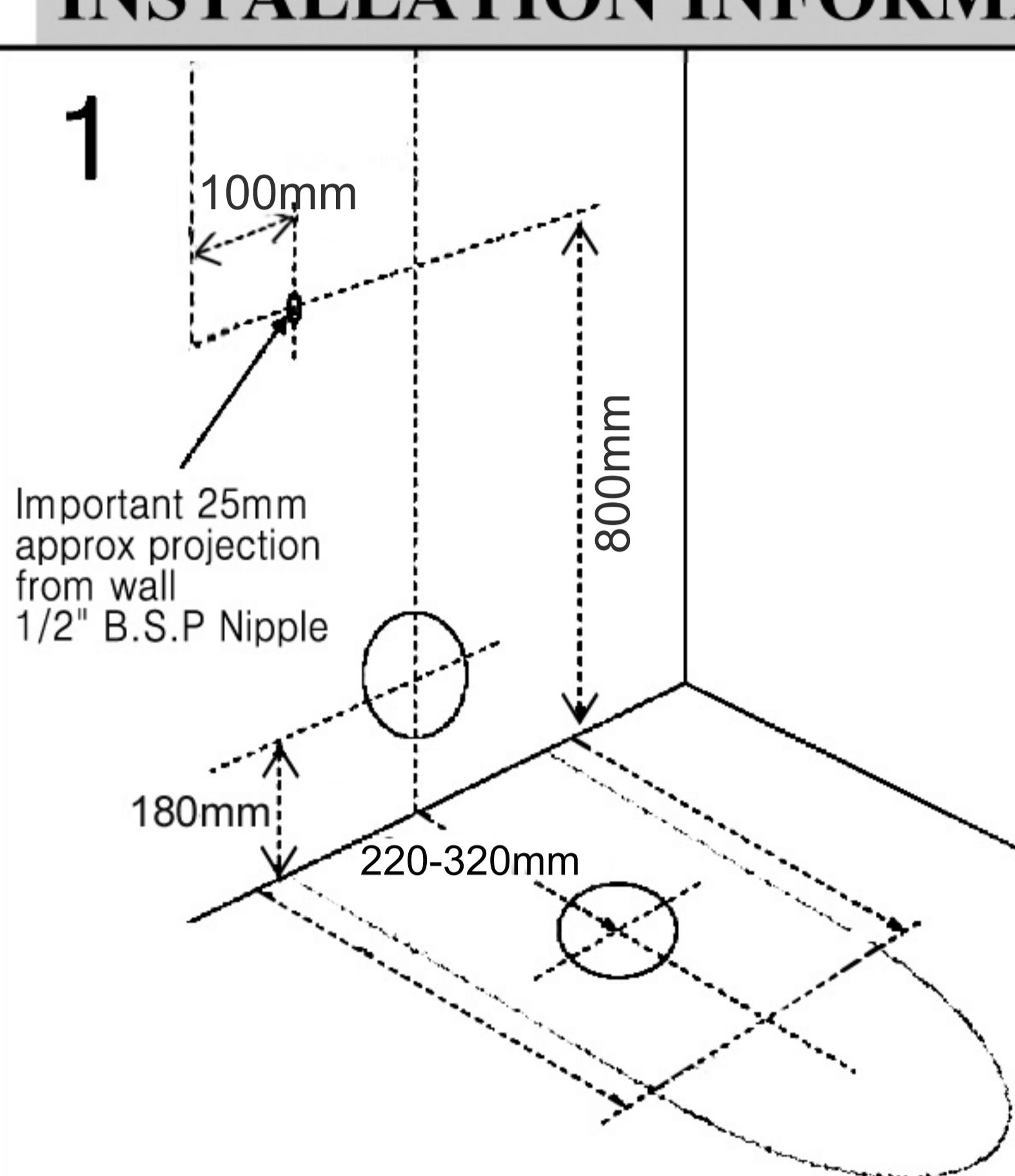
1. Rough in position of water inlet, waste outlet and floor fixing bracket holes. Ensure inlet connection extends 60mm from finished wall. Drill holes for floor fixing bracket then fix brackets to floor.
