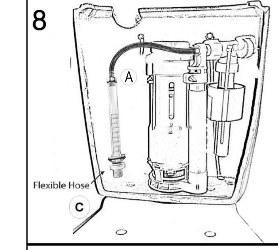
8. IF BACK INLET,SKIP THIS STEP. For Bottom(left hand) inlet connection, please connect flexible hose to plastic tube A,then complete stop tap connection to underside of cistern plug C.Fill cistern and ensure correct water level.
