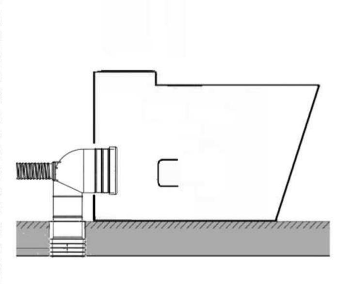
4.Align and push fully assembled toilet back to the wall
