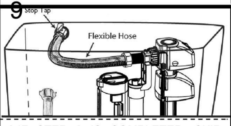
9.IF STEP 8 IS COMPLETED, SKIP THIS STEP. Fit off stop tap then connect rear water inlet valve to stop tap. Fill cistern and ensure correct water level.
