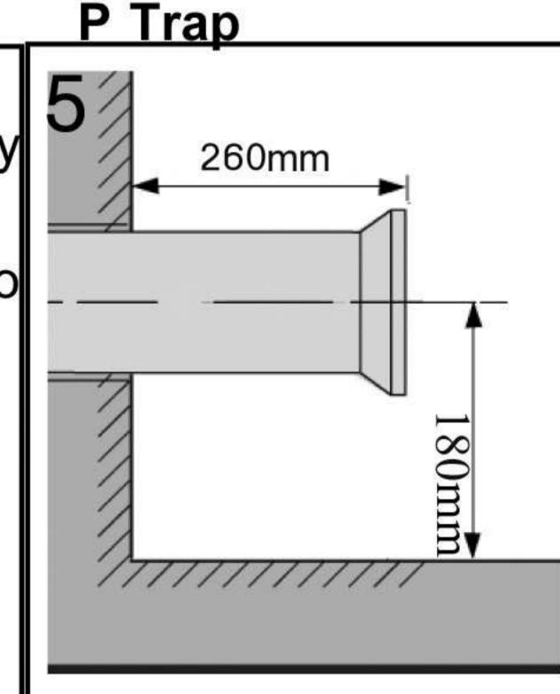
5.Set up waste pipe so that the end of the pan collar extends from the finished wall.
